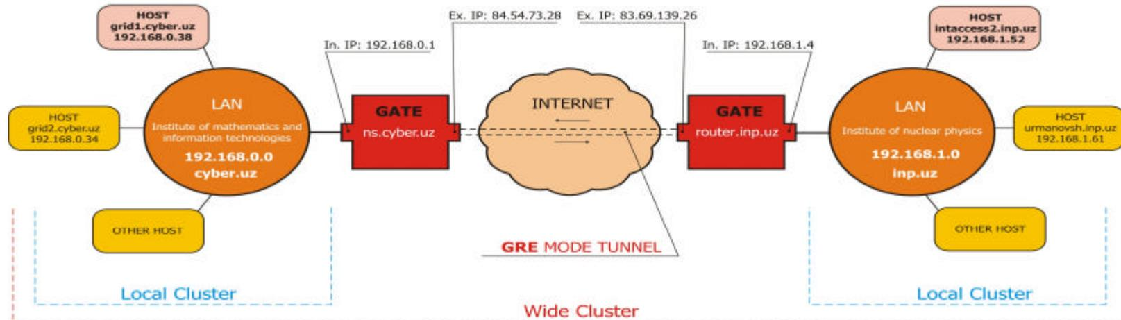
Both private networks are direct connected through the GRE mode tunnel
