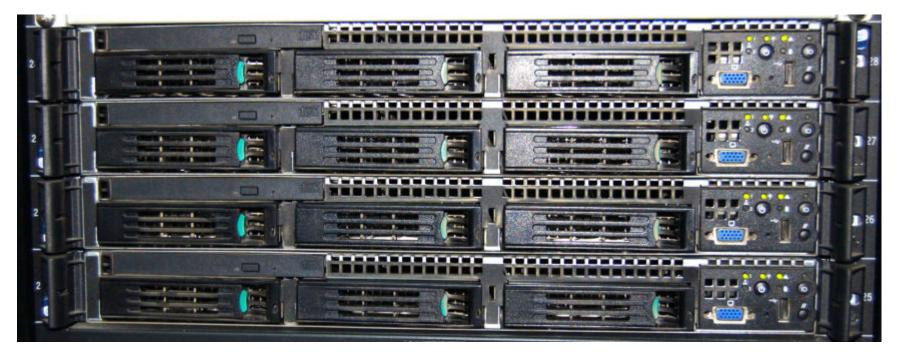
4 units with 2 double-kernel CPU in everyone. Processors Xeon 5100 with working frequency of 3 GHz, 1 Gbyte of the RAM on each kernel.
